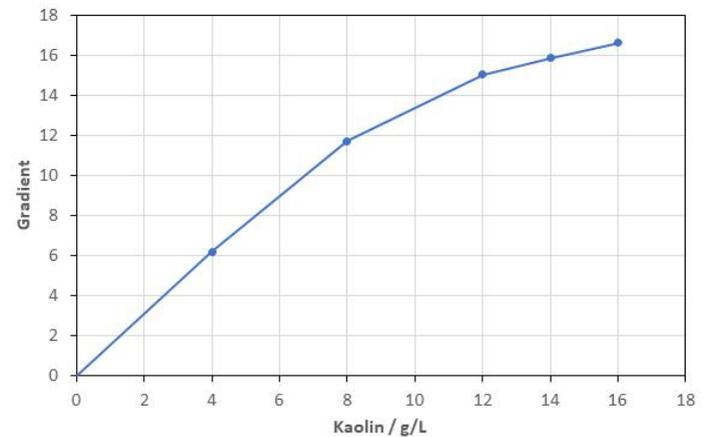
Fig. 4 Five-point SoliSense® calibration graph for kaolin.
