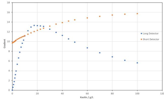
Fig. 3 Response of a SoliSense® sensor to kaolin samples.
